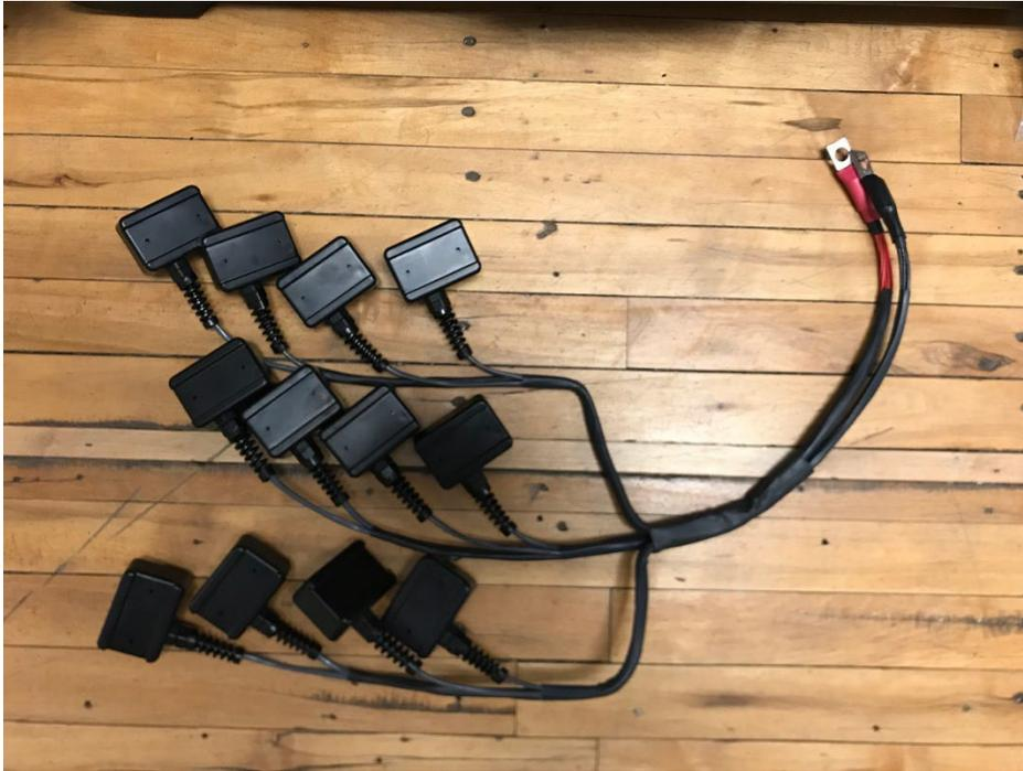
38. Place the XX90 battery harness[72996] in the case. The negative side of the harness should be attached to the DC bus closest to you. The positive side of the harness should be attached to the DC bus furthest from you. Use a 9/16" wrench, do NOT overtighten.
