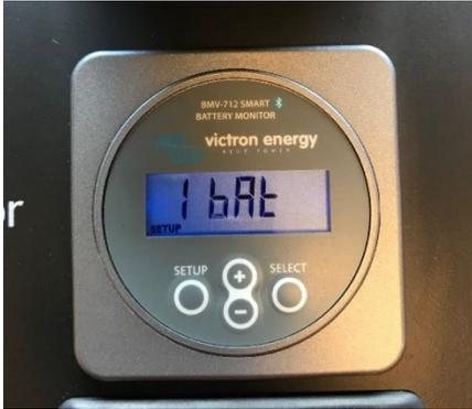
103. Press the select button on setting **number 1**, set the value of **Battery Capacity** in accordance with the battery installed in the system.
