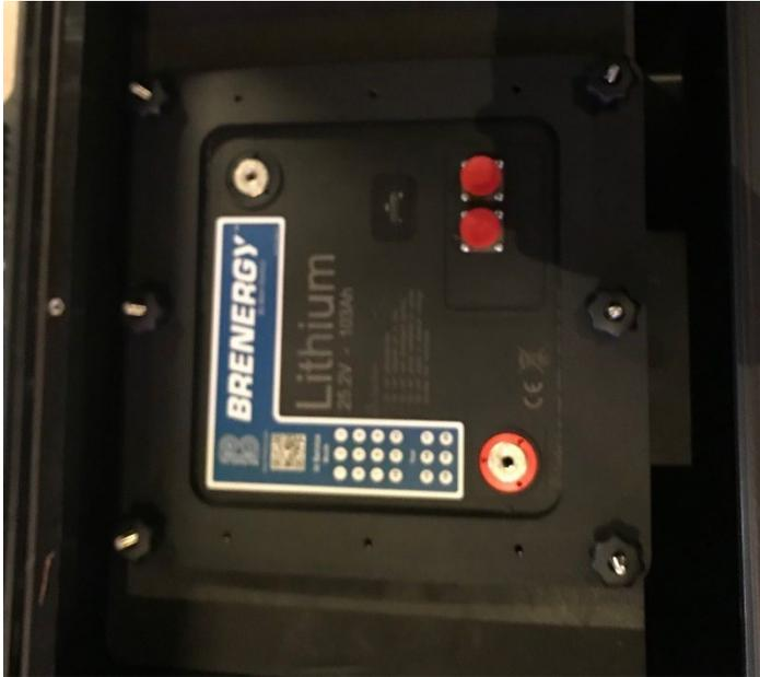
58. Attach the Battery Main leads (2 gauge) into the system.
