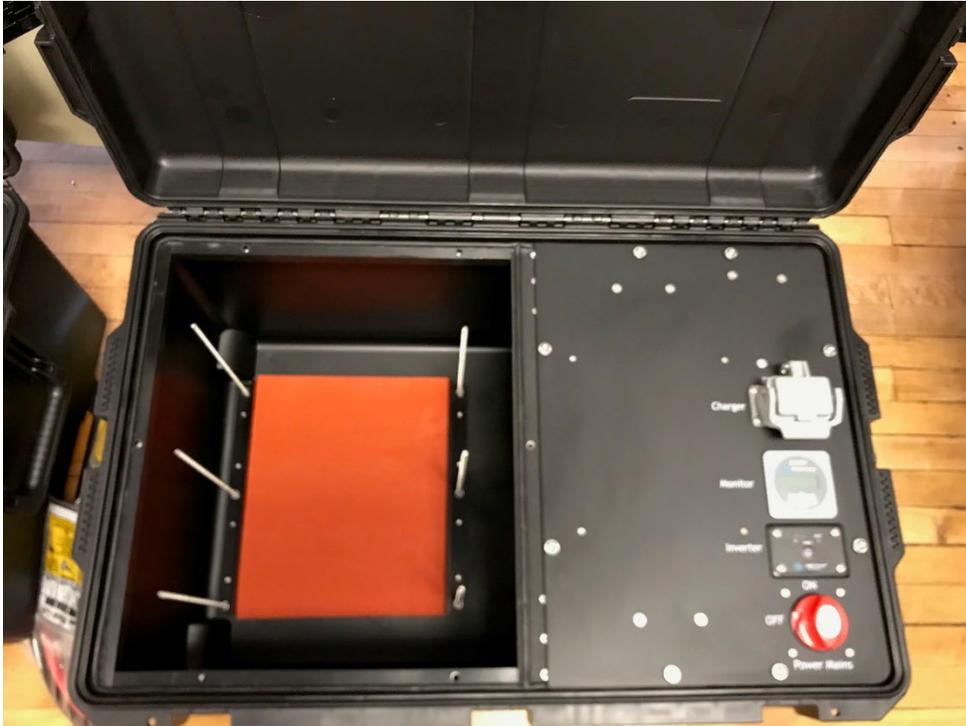
33. Install the XX90 base plate [72881] in the case. Notice the orientation of the plate, the notches circled should be facing toward the inside of the box.
