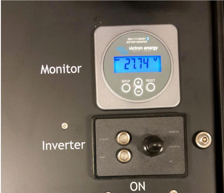
**125.** Now, turn the PPS power mains switch 90° clockwise. The switch is on when green is visible.
