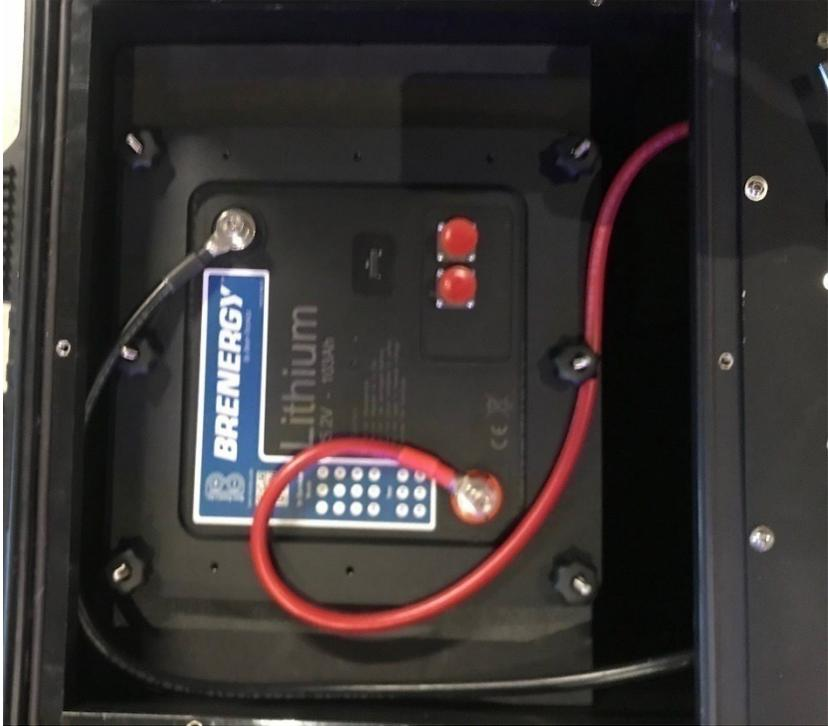
**62.** Assure all connections are tight while being very cautious of your tools. Touching multiple terminals with your tool could result in a DC short. Use a T20 torque bit to tighten.
