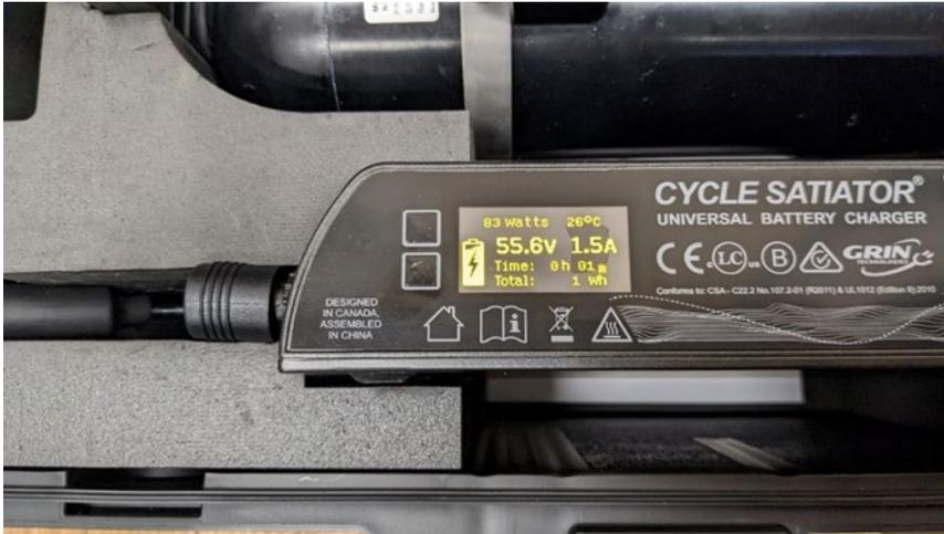
84. At this point you should see the voltage starting to increase on the battery monitor display.
