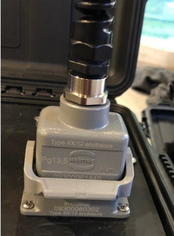
79. Plug the connector of the AC power cord into the charger's AC port.
