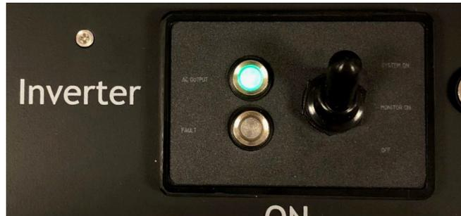
If a green light can be seen, but your equipment is not working; Check the AC output of the PPS system. Follow section 6.0 for hooking up the three outlet U.S. extension [72892]. Check for the light indicating presence of AC power.
