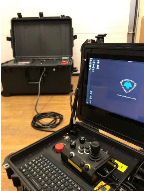
**135.** Monitor the PPS system using the Victron Connect app, or by paging through the main menu of the battery monitor on the control panel. Keep a close eye on the SOC level and the 'time to go' for a successful mission.
