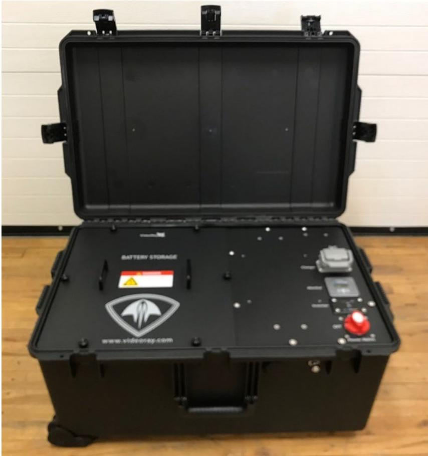
69. Whenever charging a PPS System assure that the battery storage compartment is open prior to charging.
