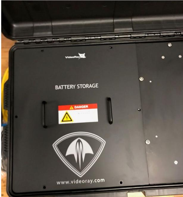
22. Reinstall the six (6) M6 male thumb screws [70256]. Tighten snugly by hand. Do NOT overtighten.
