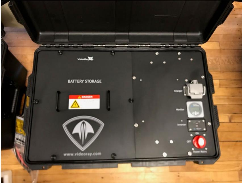
29. Assure that the power main switch is set to the “OFF” position, and that nothing is plugged into the PPS power outlet. Assure the inverter switch is set to ‘OFF’
