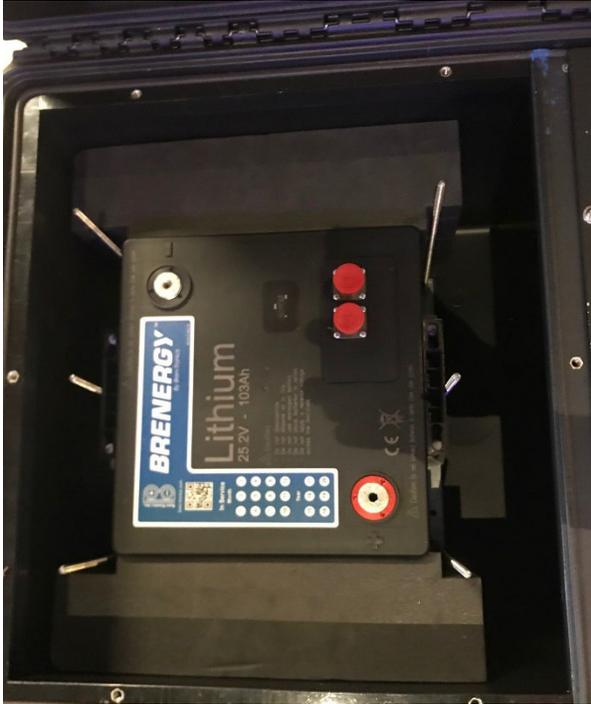
56. Install the 6T hold down plate [71605] onto the battery.
