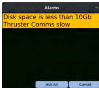
Alarms Window (Two Alarms Shown)
